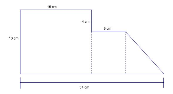
This figure can be broken into two rectangles and a triangle. Some measurements are not given but can be discovered using the measurements provided.
